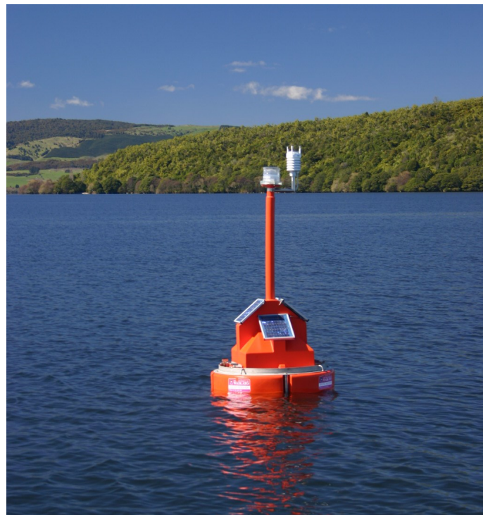
Water quality monitoring buoy on Lake Rotorua.
