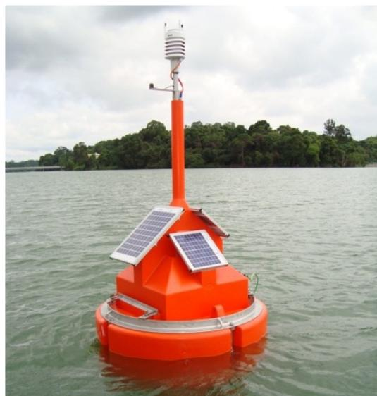
The automated monitoring buoy installed in a reservoir in Singapore.
