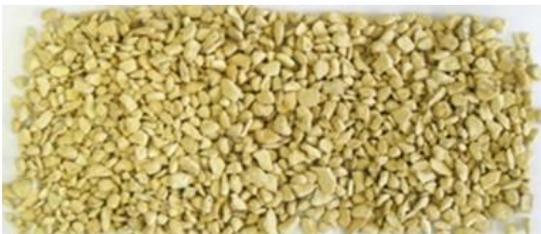
Figure 2. Modified zeolite, a sediment capping agent with a grain size of 1-3mm
